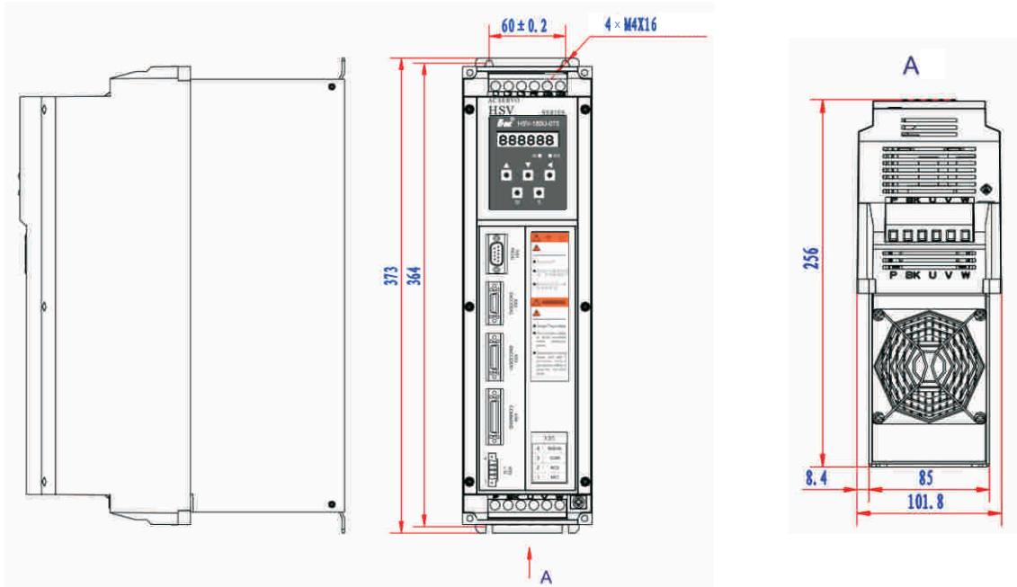
**3、HSV-180AD-,100, 150 (without auxiliary devices Unit: mm)**
