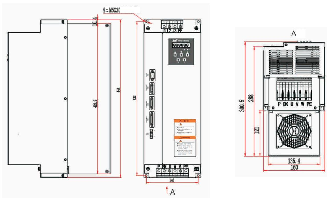
**4、HSV-180AD-100,150 (with auxiliary devices Unit: mm)**
