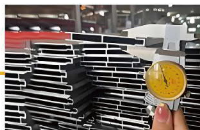
Check size, color and wall thickness
