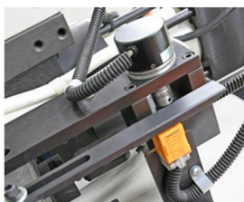
編碼器控制結幫 Encoder to control the bonding
