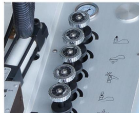
油壓壓力調整系統 Hydraulic pressure adjustment system
