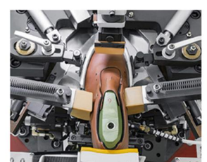
選裝輔助掃刀和輔助壓邊系統 Optional auxiliary sweeper and auxiliary flanging system
