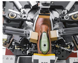
選裝輔助掃刀和輔助壓邊系統 Optional auxiliary sweeper and auxiliary flanging system
