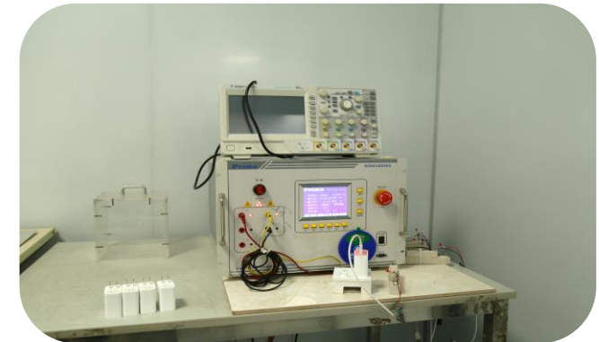
Lightning strike generator equipment
