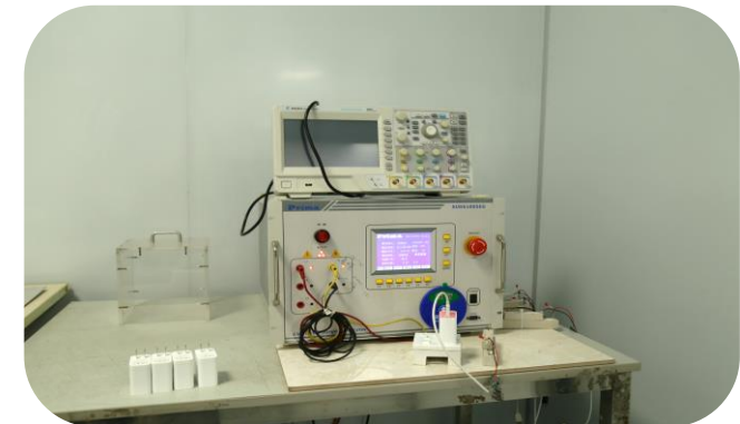
Lightning strike generator equipment
