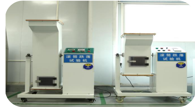
Roller drop test equipment
