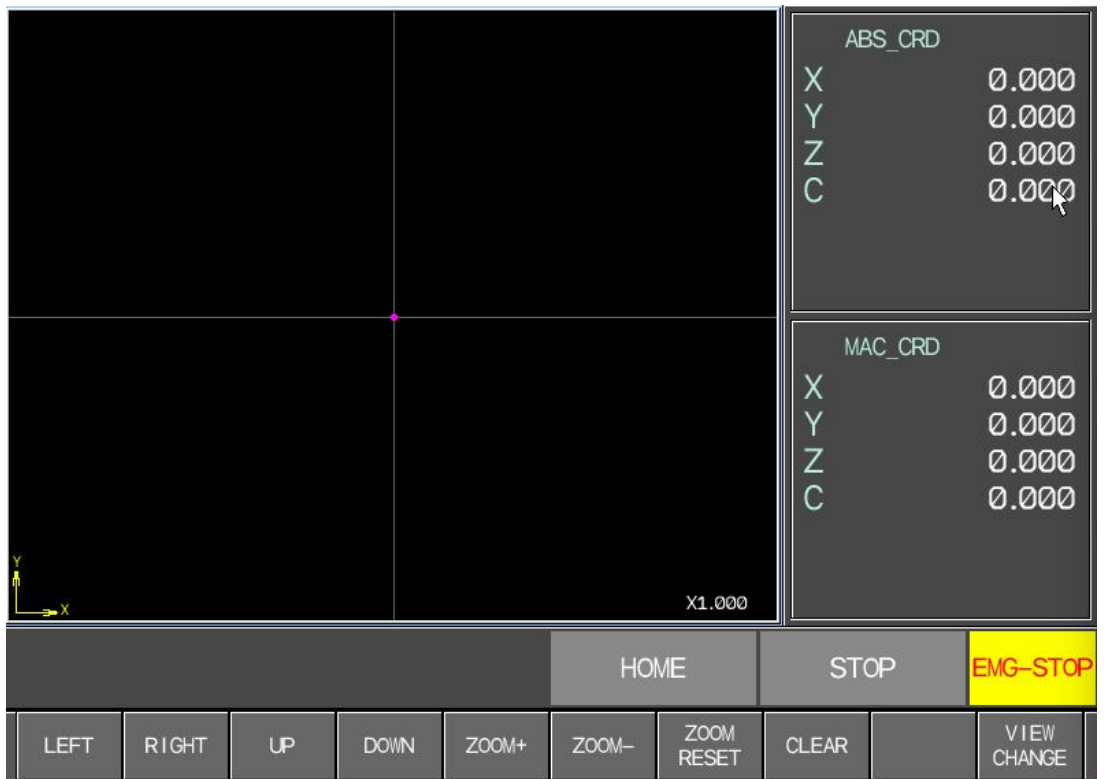
Fig. 4 -6 Simulation of the graphical track of the program
