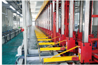
Electroplating process and quality are leading in the industry. On the fully automatic ring electroplating line with a total length of 120 meters, the surface of products is treated with five layers of electroplating to resist strong acid corrosion, which is higher than CASS test standards Unique star plating TM process.
