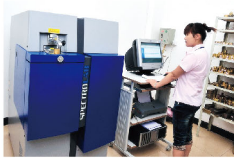
Germany imported spectrometer (copper, steel composition detection, coating thickness detection)
