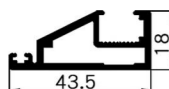
(Styles B) SK575 Name : single glass door frame (interior lock) Thickness : 2.0mm Weight : 0.599 kg/m
