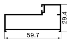
D-A546 Name : push in door Jamb Thickness : 1.1mm Weight : 0.549 kg/m
