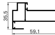
D-A554H Name : push in door Jamb Thickness : 1.2mm Weight : 0.707 kg/m
