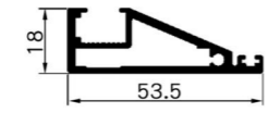
(Styles E) SK562 Name : single glass door frame Thickness : 2.0mm Weight : 0.707 kg/m
