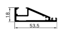
(Styles E) SK562 Name : single glass door frame Thickness : 2.7mm Weight : 0.707 kg/m
