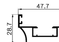
SK599 Name : double door frame Thickness : 1.0mm Weight : 0.473 kg/m
