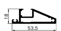
(Styles E) SK563 Name : single glass door frame Thickness : 2.0mm Weight : 0.707 kg/m
