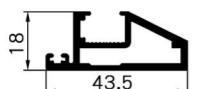
(Styles B) SK574 Name : single glass door frame (interior lock) Thickness : 2.0mm Weight : 0.599 kg/m
