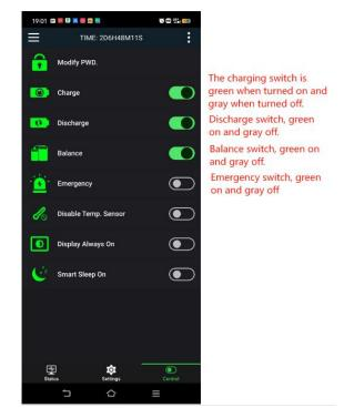
7.6.1 Charging switch: used to control the charging switch of the protection board to turn on or off.
