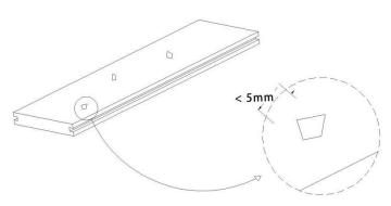
Wood dust or impurity: one piece has more than 3 impurities which are larger than 5mm
