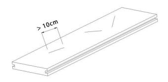
Scratch mark: one piece has more than 3 scratches which are longer than 10cm
