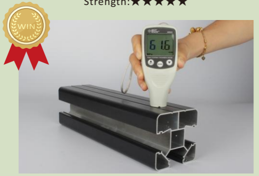
Coating thickness: 61.6um Durability: ★★★★★
