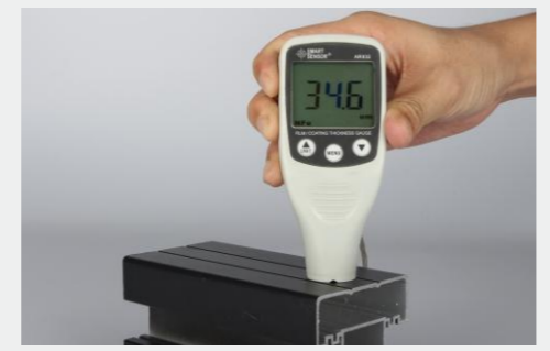
Coating thickness :34.6um Durability:★
