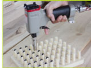
Step2 Put the nose on the studs
