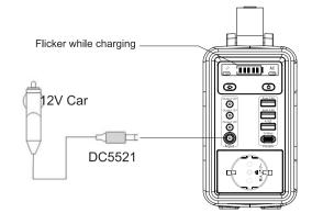
A. Plug the original car charger into the cigarette lighter socket of your 12V car, and then plug into the ACinput port of the machine.
