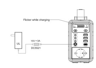
Plug the original adapter into the machine's AC input port and you will see the battery indicators on the screen blink.
