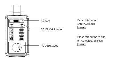
A. Press the power button to enter AC mode. Plug the power cable of AC appliance B. Make sure the power of the connected AC appliance is less than 200W.
