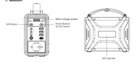
A. Long press the power button for 3 secs to turn the machine on. Press the button again to turn on the AC function, press again to turn off. B. Long press the button for 3 secs again to turn off the machine.
