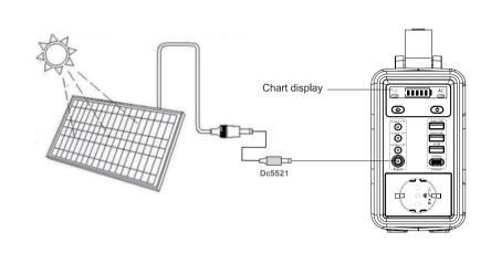
A.Place your solar panel where it will get as much strong direct sunlight as possible. B.Connect the output port of the solar panel with the input port of the product to start charging. You will know the product is being charged when the LCD display indicators blink. The product is fully charged when all battery indicators stop blinking and remain solid.
