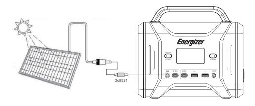
A.Place your solar panel where it will get as much strong direct sunlight as possible. B.Connect the output port of the solar panel with the input port of the product to start charging. You will know the product is being charged when the LCD displays the charging percentages on the screen. The product is fully charged when displays 100%.
