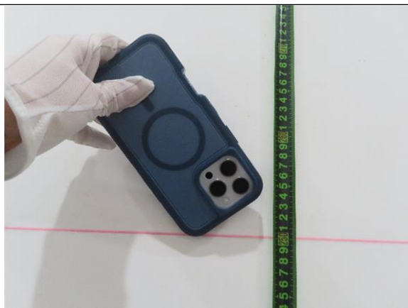
During test-Drop corner
