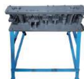
▼ punching machine (door panel frame hole) (PT-PM-001)
