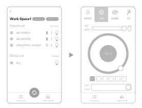
Click on the device name to enter the control interface to control your lighting
